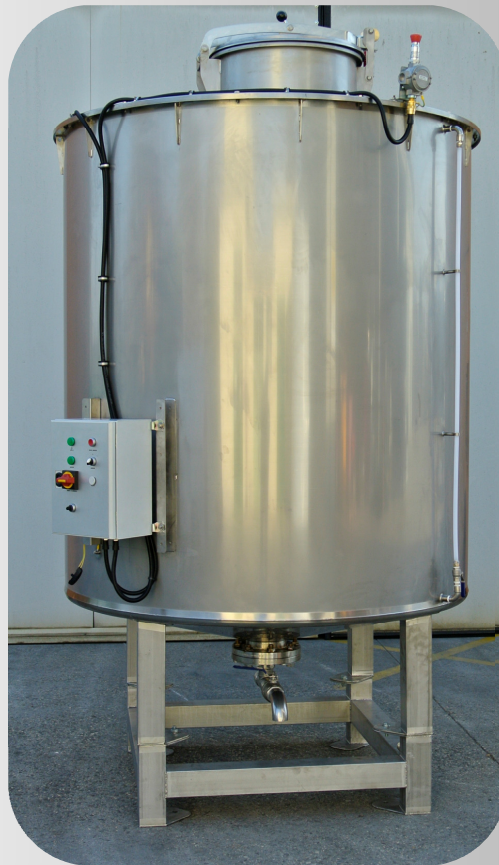
Mixing tank for wax
